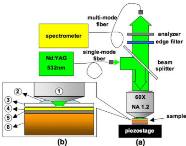
**Figure 1.** (a) Schematic diagram of the experimental setup. (b) Zoom-in view of the objective lens and the sample. Water immersion objective lens (1) that is immersed in water (2) is used to focus the excitation laser to the sample. Points (3)–(6) correspond to the cover glass, the silver coating; the strained-Si layer and the substrate, respectively. This figure is available in colour online at [www.interscience.wiley.com/journal/jrs](http://www.interscience.wiley.com/journal/jrs).
